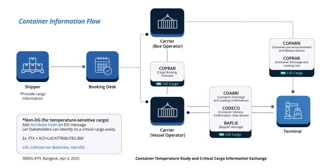
Proposed container information flow for temperature-sensitive cargo leveraging SMDG code.
